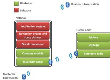
Figure 1: System architecture.
