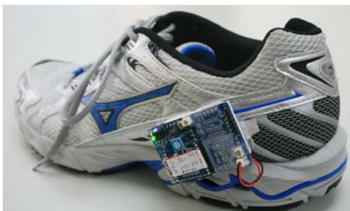
Figure 5: Intelligent shoes. A sensing module is attached onto the side of the shoe. The sensing values will transfer wirelessly through the XBee module.
