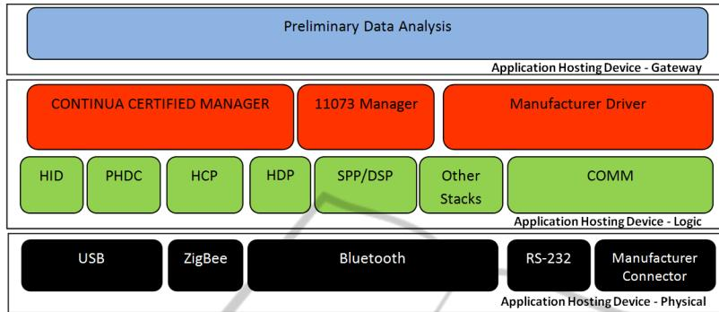
**Fig. 2.** Application Hosting Device Stack.
