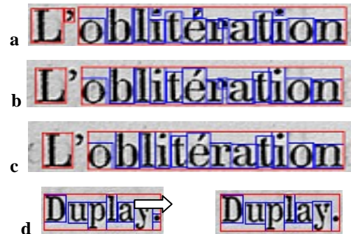
Figure 3: a) Original comps b) After Pass1 c) After Pass 2 d) Pass 3 demonstration, bounding box of the punctuation mark is removed (Khurshid, 2008).
