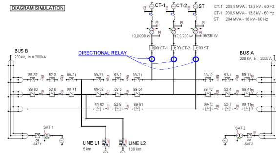
Figure 6: Substation model used in the simulation faults.
