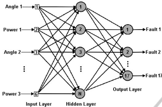
Figure 5: MLP structure used in the Expert System.
