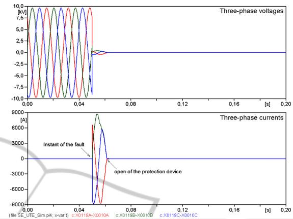
Figure 9: Voltage and currents on out CT2 generator with fault of the circuit breaker 52-4.
