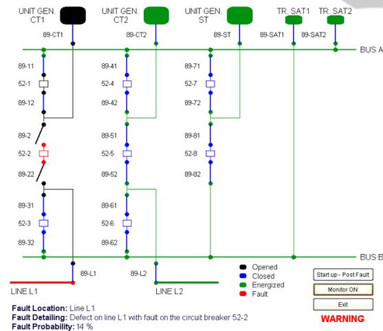
Figure 8: Software interface shows fault at Line L1.
