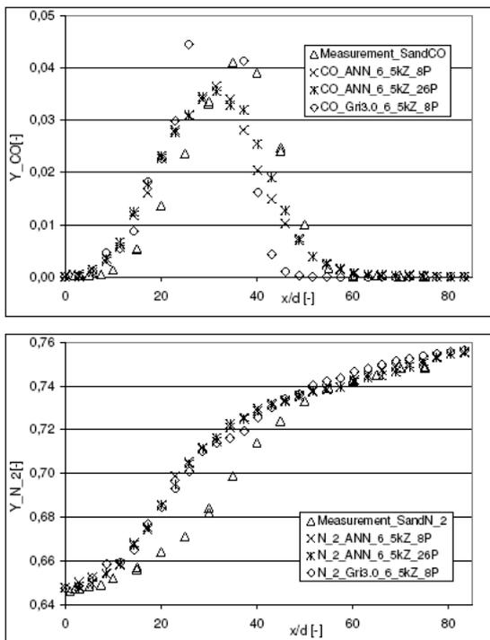
Figure 6: Comparison of measurements, ANNs and ODE system simulation solutions of carbon monoxide and nitrogen.
