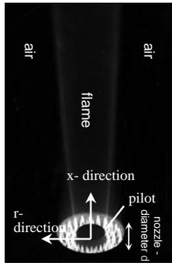
Figure 1: Picture of the Flame (Sandia, 2003) with description (added).
