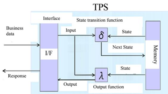
Figure 1: Structure of the TPS.
