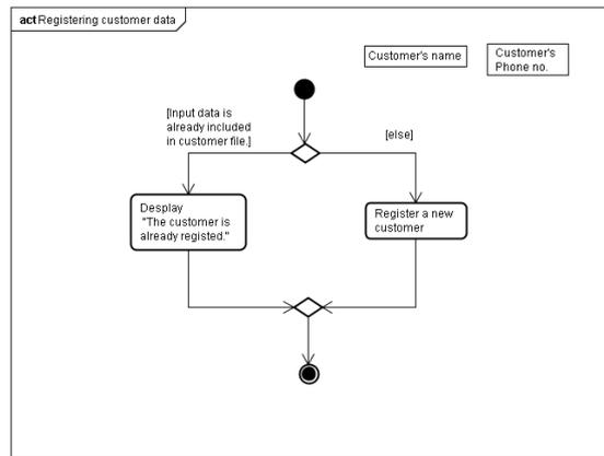
Figure 8: Activity diagram for registering customer data.
