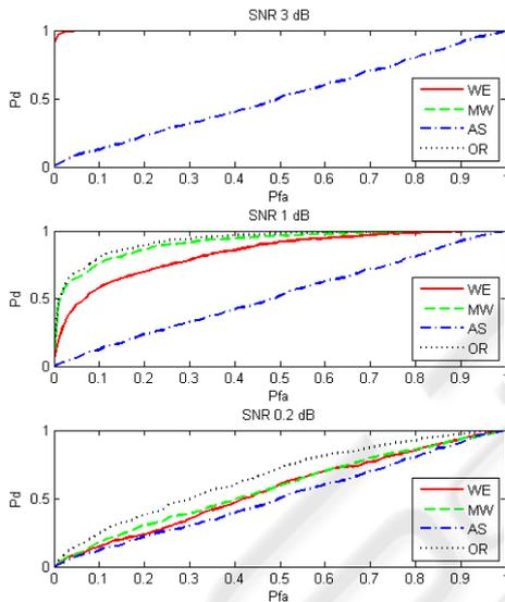
Figure 5: ROC curves for three investigated detectors – Welch (WE), MultiWindow (MW), key feature AS, together with OR fusion of Welch’s and Multi Window in various SNR.
