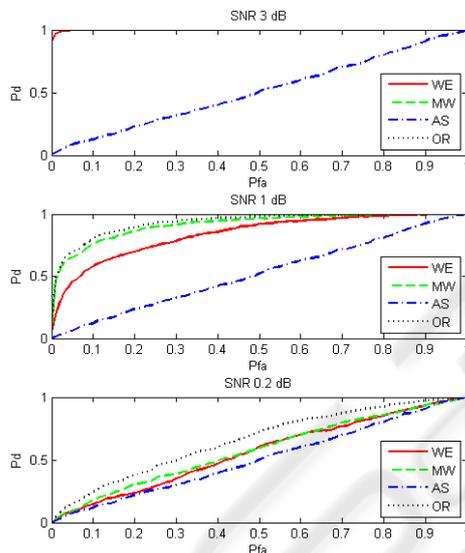
Figure 5: ROC curves for three investigated detectors – Welch (WE), MultiWindow (MW), key feature AS, together with OR fusion of Welch’s and Multi Window in various SNR.
