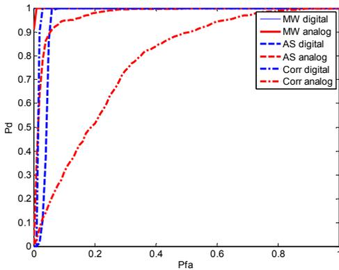
Figure 4: ROC curves for Multi Window (MW), key feature AS and correlation (Corr) detectors for both digital and analog TV signals sampled at DVT-T receiver IF output.
