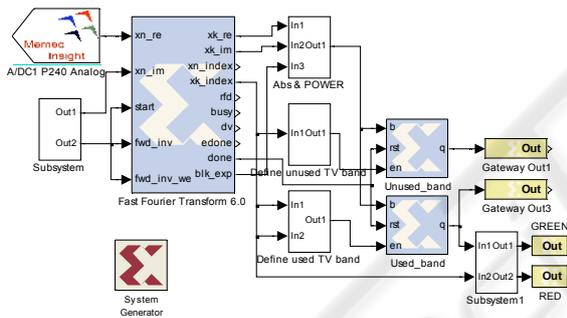
Figure 2: Simplified block diagram of the FPGA implementation (created in Xilinx System Generator).
