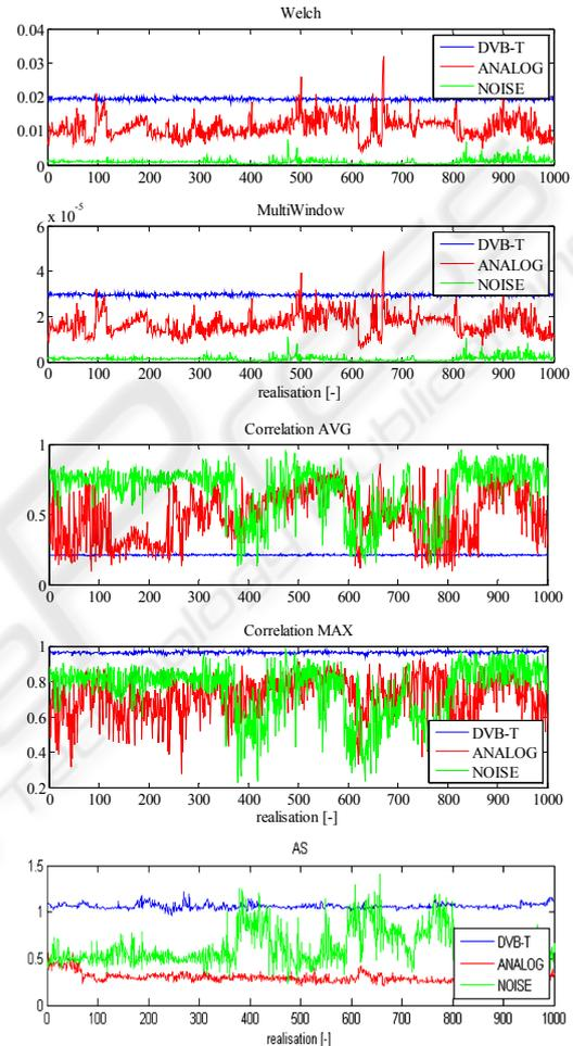
Figure 3: Test statistics for various detector types . From top to bottom: Welch periodogram, MultiWindow, Correlation (average value), Correlation (max value), key feature AS.
