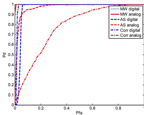
Figure 4: ROC curves for Multi Window (MW), key feature AS and correlation (Corr) detectors for both digital and analog TV signals sampled at DVB-T receiver IF output.
