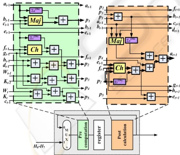
Figure 5: Partially unrolled operation block with pre-computed values.
