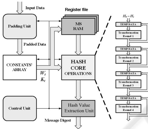
Figure 1: SHA-256 hash core architecture with 4 pipeline stages.
