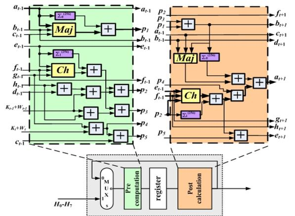
Figure 6: Partially unrolled operation block with pre-computed values for SHA-256 with pre-fetching of  $W+K$  values.
