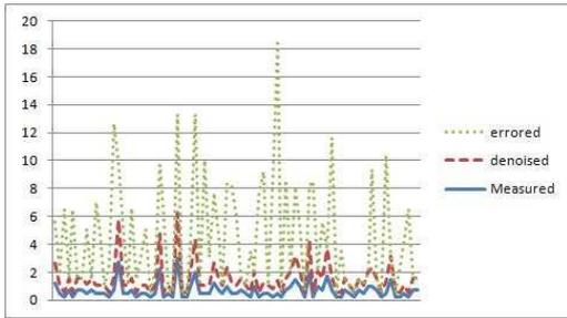
Figure 3: Comparison of measured, errored, and denoised link delays on Link2.
