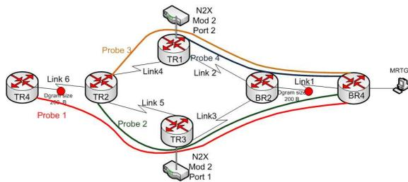
Figure 1: Testbed Setup with a mixture of extended pings and N2X traffic.
