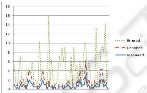
Figure 5: Comparison of measured, errored, and denoised link delays on Link4.
