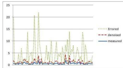
Figure 2: Comparison of measured, errored, and denoised link delays on Link1.
