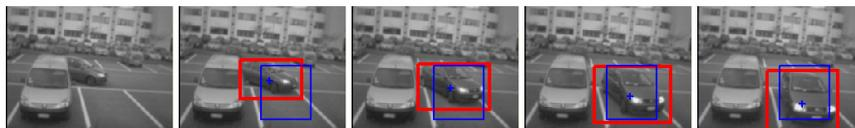
**Fig. 4.** Car detection and analysis of parking lot occupancy status.
