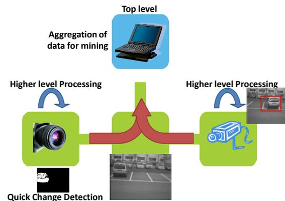
**Fig. 2.** Architecture of the hierarchical levels of detection, in a car detection case study.
