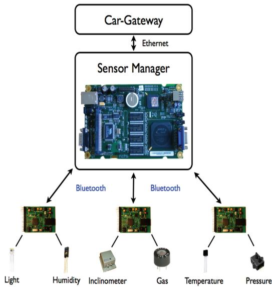
Figure 2: General architecture of the sensor network.
