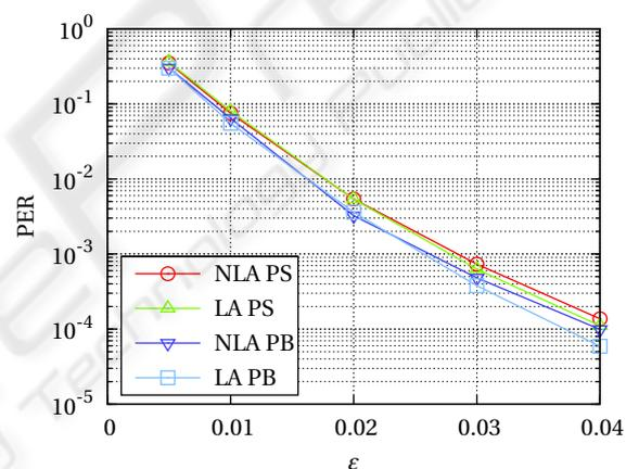
Figure 9: Performance for MAP soft-decision decoder for static binary model with  $M = 256$  and  $E_b/N_0 = 5.5$  dB; without look-ahead (NLA) and with look-ahead (LA); and with  $P(\mathbf{t})$  adjusted every symbol (PS) or every bit (PB).
