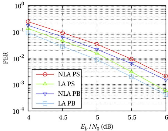
Figure 6: Performance for MAP hard-decision decoder for static binary model with  $M = 256$  and  $\epsilon = 0.185$ ; without look-ahead (NLA) and with look-ahead (LA); and with  $P(\mathbf{t})$  adjusted every symbol (PS) or every bit (PB).
