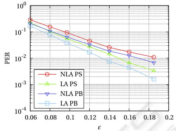
Figure 8: Performance for MAP hard-decision decoder for static binary model with  $M = 256$  and  $E_b/N_0 = 5.5$  dB; without look-ahead (NLA) and with look-ahead (LA); and with  $P(\mathbf{t})$  adjusted every symbol (PS) or every bit (PB).
