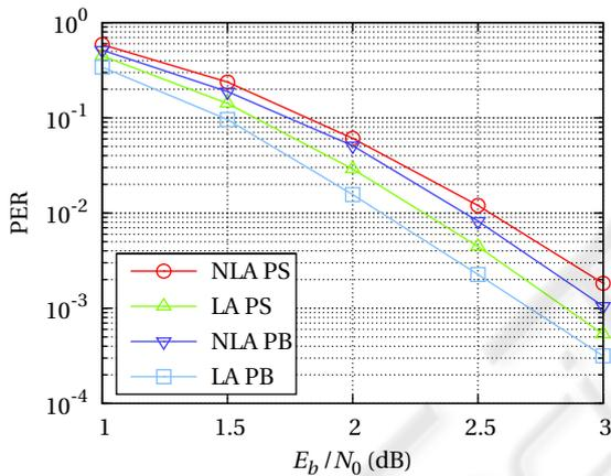
Figure 7: Performance for MAP soft-decision decoder for static binary model with  $M = 256$  and  $\epsilon = 0.185$ ; without look-ahead (NLA) and with look-ahead (LA); and with  $P(\mathbf{t})$  adjusted every symbol (PS) or every bit (PB).
