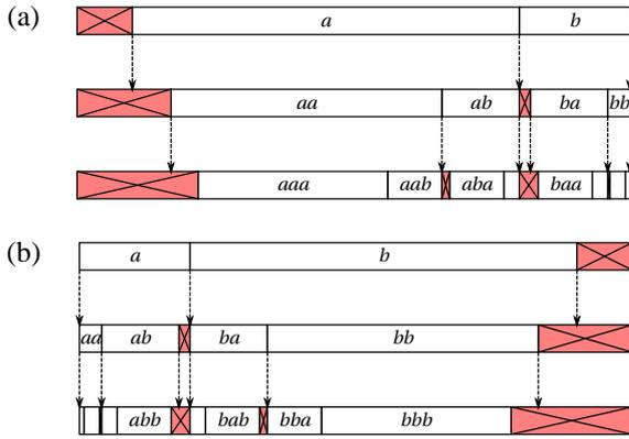
Figure 3: Forbidden gaps after three stages when placed to reduce error-detection delay for (a)  $P(a) > P(b)$  and (b)  $P(a) < P(b)$ .
