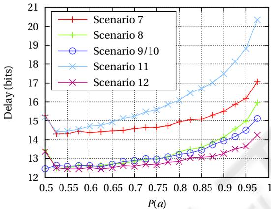
Figure 5: Error-detection delay for adaptive source model with a code rate of 8/9.
