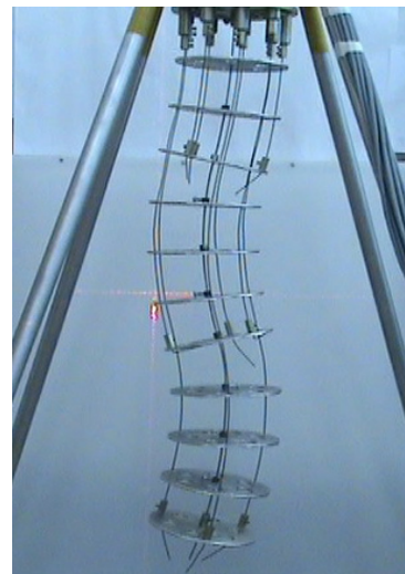
Figure 3: The assembly of the robotic system with the baggy vertebral unit.
