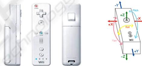
Figure 1: Wiimote and its accelerometer axes.
