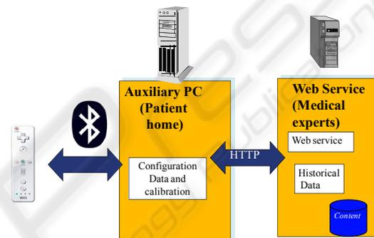
Figure 2: Architecture of the fall detection system.
