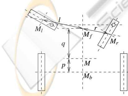
Figure 4: Mass distribution to castor and differential drive wheels.
