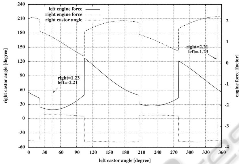
Figure 5: Castor angles with maximal differential drive load.
