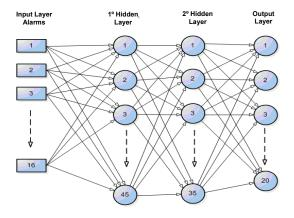
Figure 2: Feeder bay ANN with multiple neurons in the output.
