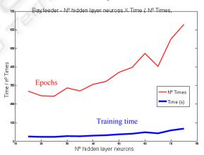
Figure 9: Hidden layers neurons X time & epochs for feeder bay and one output neurons ANN.
