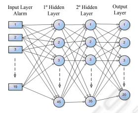
Figure 4: Capacitor bank bay ANN with multiple neurons in the output.
