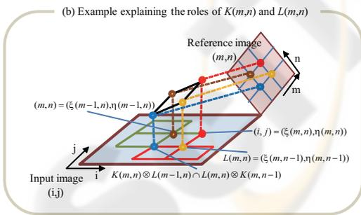
Figure 4: One case (linear matching) among the possible cases for optimal matching of local images, which include many different cases of nonlinear optimal matching of local areas.
