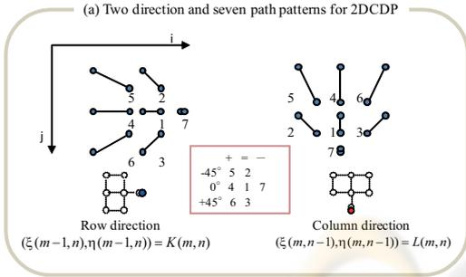
Figure 3: Two directions and seven paths for selecting optimal path to accumulate value.
