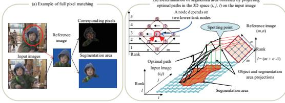
Figure 2: Full pixel matching overview. (a) An example of full pixel matching; (b) Optimal paths are able to explain a 3D space  $(i, j, l)$  in the input image.  $l$  is the rank used in the expression  $l = m + n - 1$ .
