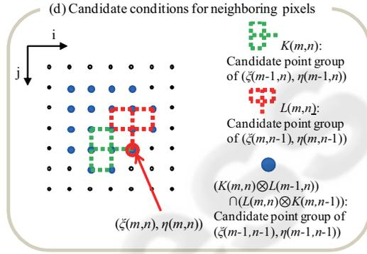
Figure 6: Each  $i$  and  $j$  direction can connect seven candidate pixels as (a) and (c). 2DCDP selects the node that has a minimal accumulation value from among these paths, but a node has depending on only two lower-rank nodes.
