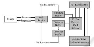
Figure 9: Authentication system using multiple nVidia CUDA enabled video cards.
