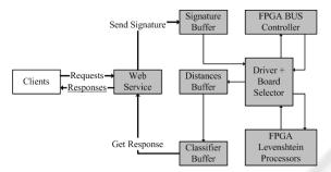
Figure 7: Authentication system using multiple FPGA boards.
