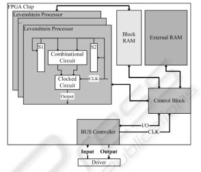
Figure 6: General architecture of a system performing multiple Levenshtein comparisons on a FPGA board.
