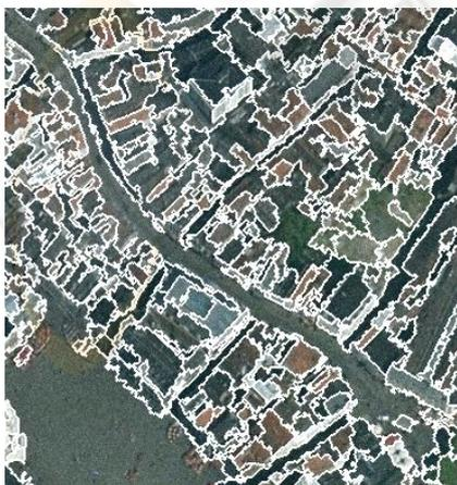
Figure 2: Mean shift segmentation results on a zoom of the image of figure 1.
