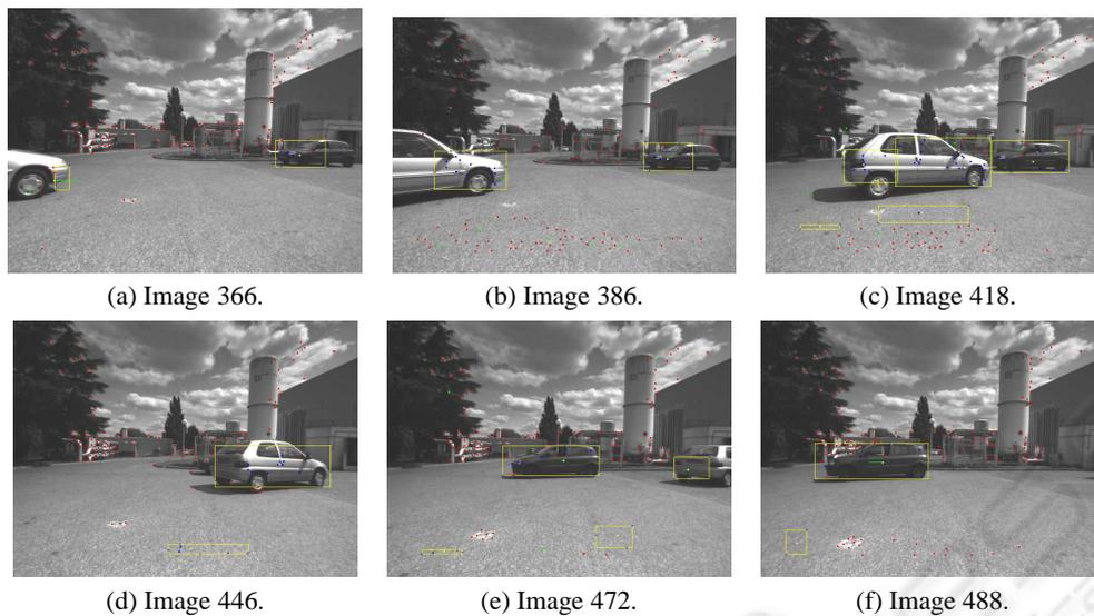
Figure 2: Detection clustering and tracking of moving objects during robot navigation. Top row: Detection and tracking of right side car  $O_1$  and left side car  $O_2$ . Second row:  $O_1$  and  $O_2$  cross front visual field of robot until  $O_2$  is out of image.
