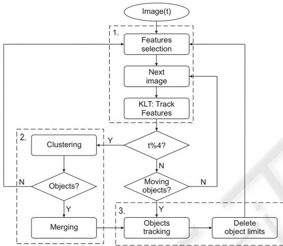
Figure 1: Algorithm to detect and track multiple moving objects.
