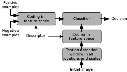
Figure 2: The “descriptor/classifier” framework principle.
