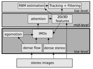
Figure 1: Illustration of the architecture presented in this paper.
