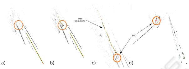
Figure 8: Illustration of a) the reconstructed road structure, b) and c) trajectories for the ego- and IMO-motion, and d) the reconstructed 3D model of the car with the lane structure.
