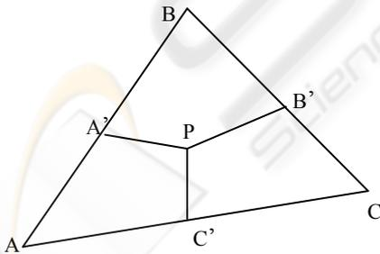
Figure 4: Split a triangle into quadrilaterals.
