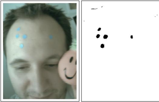
Figure 4: Image of volunteer with blue markers on his forehead (left), and the result of transforming the image to the HSV color model and thresholding the H-channel (right).
