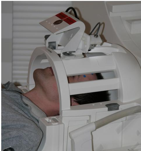
Figure 2: Camera mounting on top of Siemens Trio Head Coil.
