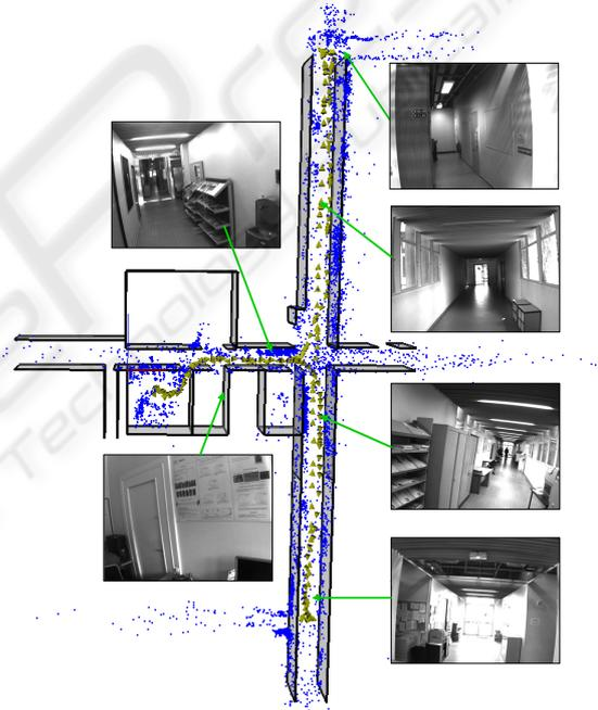
Figure 2: The database used for the LKE algorithm. This Structure from Motion point cloud comes from the LUKE algorithm. The drift is *a posteriori* corrected with the procedure described in (Lothe et al., 2009).
