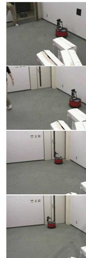
Figure 8: A dynamic environment. After the door to the corridor is closed, the robot recognises that the door is a part of wall and find a path to the left.
