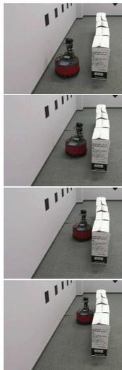
Figure 6: Experimental result for mobile robot navigation using hierarchy of plane segments. The robot passes through the corridor, whose width is about the twice of the width of the robot, without collision to the wall of the corridor.
