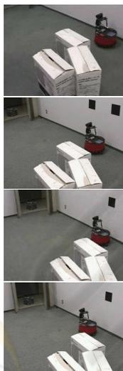
Figure 7: A sparse real environment. Although obstacles are large, the robot decides a straight path in a sparse environment.
