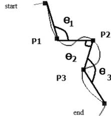
Figure 2: Break down of a curve segment in order to calculate its fitness value.
