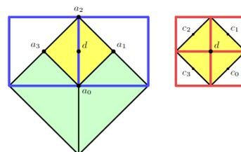
Figure 1: A diamond  $d$  (yellow) is shown with its ancestors (left) and its children (right) (Hwa et al., 2004). The green ancestor is  $a_0$ , the two parents are  $a_1$  and  $a_3$  (blue outline).  $d$ 's children are  $c_{0..3}$  (red). Note that the orientation is rotated by  $45^\circ$  each level.
