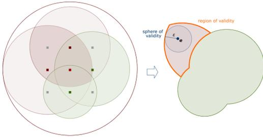
Figure 4: Red represents the spheres of the active vertices and green those of the inactive vertices with respective *region of validity* and *sphere of validity* for a view-point.
