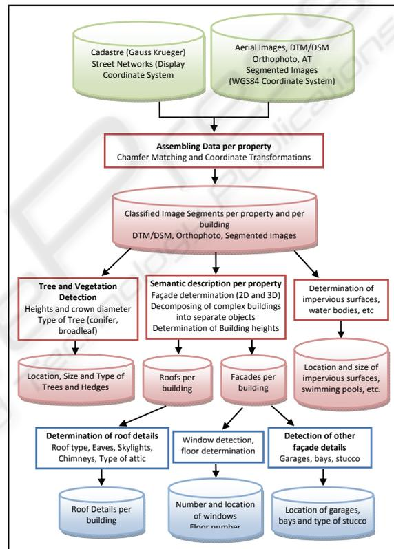
Figure 3: Diagram of the proposed work flow to characterize real properties from aerial images and associated cadastral data.
