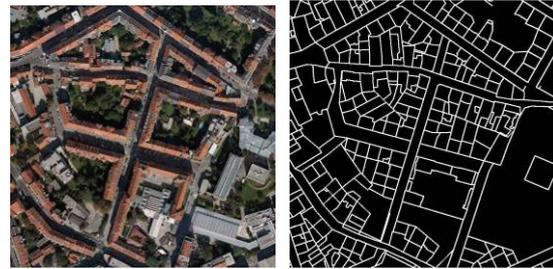
Figure 2: Left is a True Orthophoto of the city of Graz, 400 m \* 400 m, at a ground sampling distance of 10 cm. Right is a cadastral map of Graz [Courtesy BEV-Austria].
