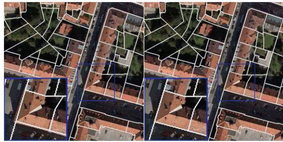
Figure 5: Overlaying the cadastral map over the orthophoto will leave some small errors that need to be found and removed. Left after step1, right after step 2.
