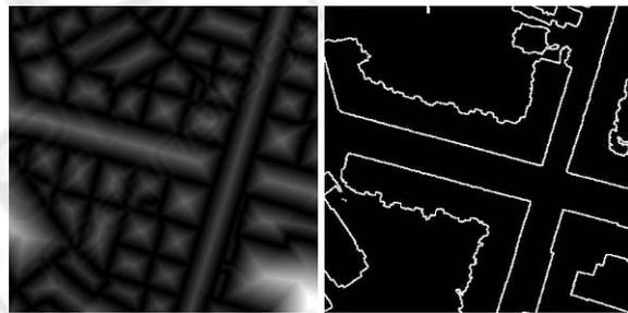
Figure 6: Cadastral raster distance image (left) and edge image (right) for a chamfer match.
