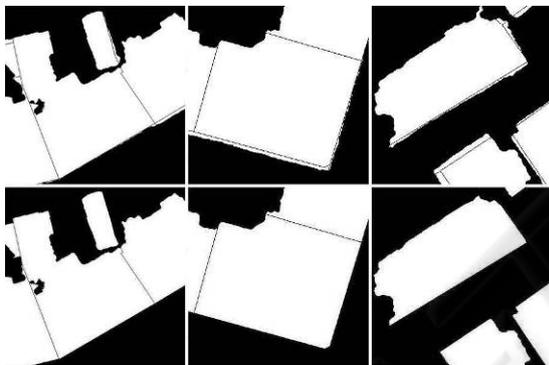
Figure 8: Overlay of segmented image and cadastre for areas in Figure 8. Above is with the discrepancies due to roof eaves and façade detail, below is a manually cleaned-up version.
