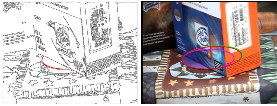
Figure 4: Left: Edge image containing a small elliptic edge segment (red). Right: Ellipses fitted to 155 edge points overlaid on the original image. From inner to outer are the ellipses computed by least squares (pink), Taubin method (blue), proposed method (red), and maximum likelihood (green). The proposed and Taubin method compute almost overlapping ellipses.
