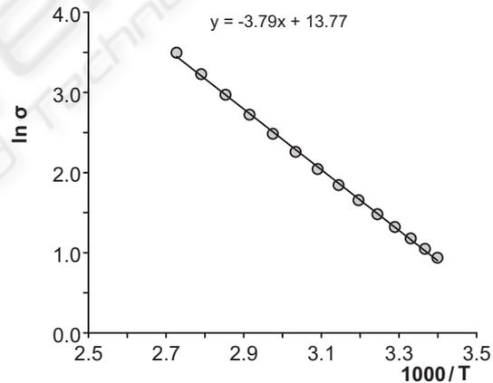
Figure 4: Plot of  $\ln \sigma : 1000/T$  for the calculation of the energy gap of Ge crystals.
