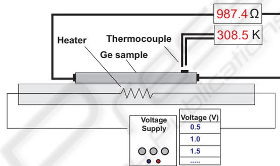
Figure 3: Typical circuit with a Ge crystal.
