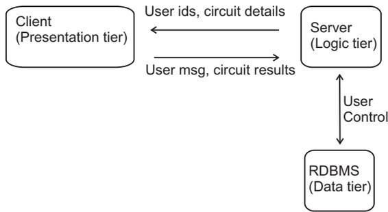
Figure 2: System architecture.
