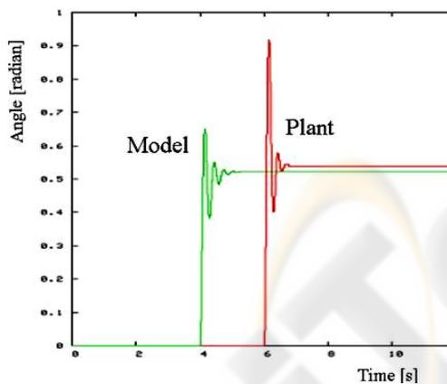
Figure 5: Step response by PID controller.
