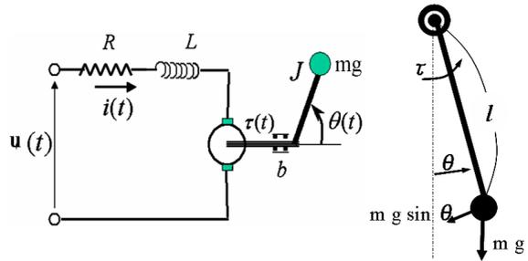
Figure 3: DC motor and a pendulum.
