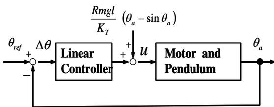
Figure 4: Real time input linearization.
