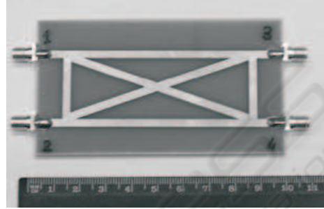
Figure 2: Picture of the constructed coupler.
