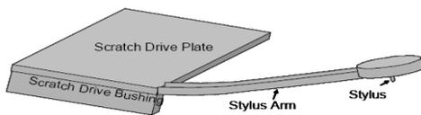
Figure 1: Illustration of MEMS Micro-robot (Donald et al., 2006).
