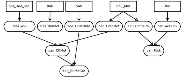
Figure 2: A capability graph. Rectangles are components, and rounded rectangles are capabilities (6 basic and 3 composed capabilities).
