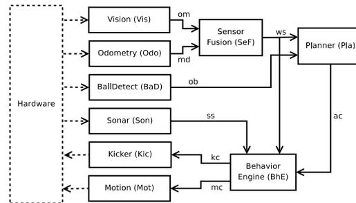
Figure 1: Architecture of a control system for an autonomous soccer robot. Connections depict data flows.
