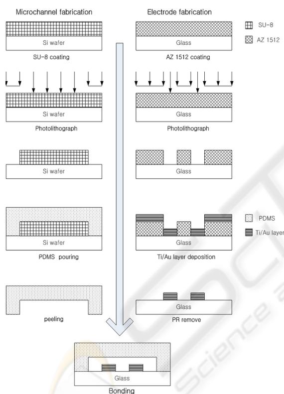
Figure 1: Fabrication process for Microchip.
