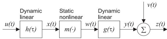
Figure 1: The Wiener-Hammerstein model.
