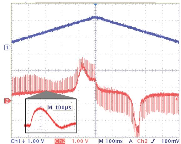
Figure 6: Time domain potentiostat response to a DAC generated cyclic voltammetry signal.
