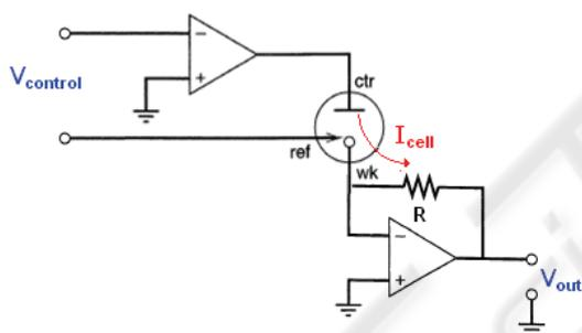
Figure 1: Standard potentiostat topology with inverting control amplifier and transimpedance current measurement.
