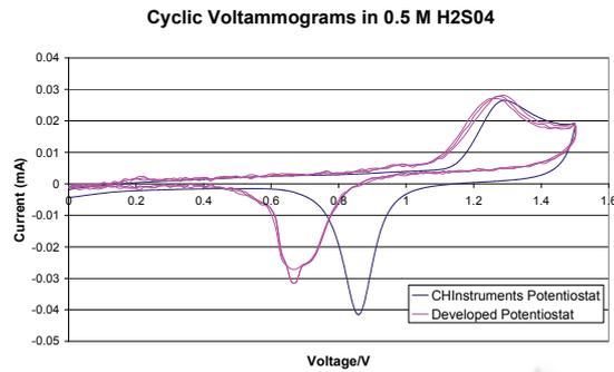
Figure 5: Cyclic Voltammogram for the developed potentiostat and a CHInstruments Potentiostat in 0.5M H<sub>2</sub>SO<sub>4</sub>.
