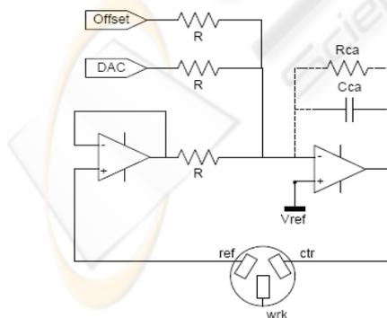
Figure 3: Potentiostat sensor control circuit with input stimulus voltage from DAC and connections to sensor.
