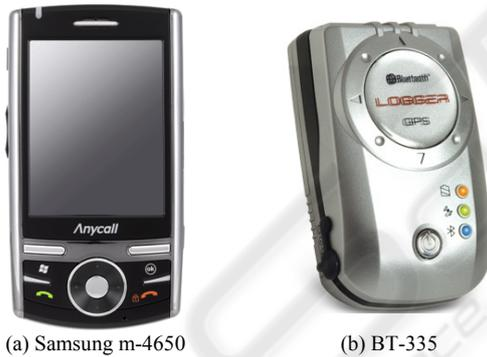
Figure 5: Smartphone (a) and portable GPS (b) used for data collection.
