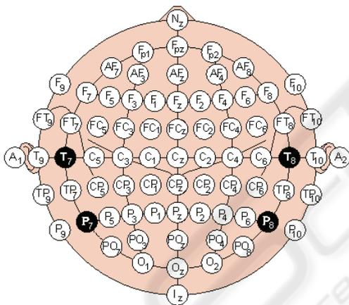
Figure 2: Position and names of the electrodes.
