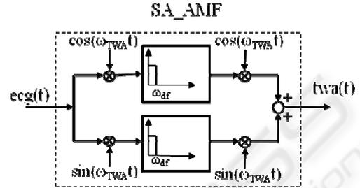
Figure 2: Signal-adapting AMF implementation (SA\_AMF).
