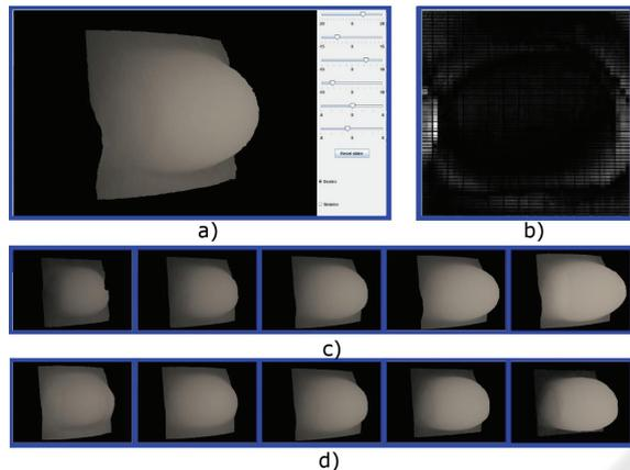
Figure 4: a) The graphical user interface of our JAVA application; b) Typical reconstruction error distribution; c) Variations induced by the first parameter; d) Variations induced by the second parameter.
