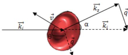
Figure 1: Single scattering event between a photon and a moving scatterer, in this case a red blood cell.  $\vec{k}_i$  and  $\vec{k}_s$  denote the incoming and scattered wave vectors, and  $\alpha$  is the angle between the two.  $\vec{v}$  is the velocity vector of the red blood cell.  $\vec{q}$  is the difference between  $\vec{k}_i$  and  $\vec{k}_s$ .  $\theta$  is the angle between  $\vec{q}$  and  $\vec{v}$ .
