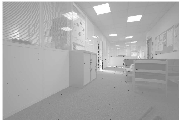
Figure 3: Corridor scene and flies resulting of one particular run of the Fly algorithm, projected on the corridor scene (printout contrast has been reduced in order to enhance the visibility of flies).
