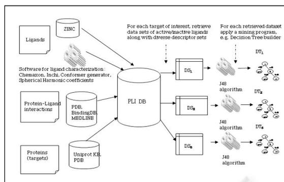
Figure 2: KDD process for designing knowledge-based filters in a virtual screening context.
