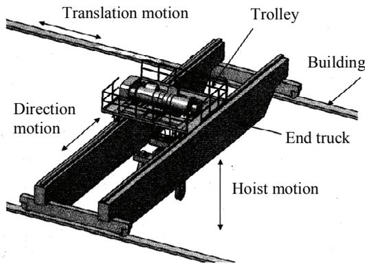
Figure 2: A typical overhead crane.
