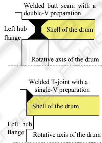
Figure 4: Two categories of welded seams.
