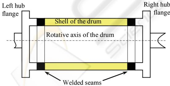
Figure 3: Schematic design of the drum.
