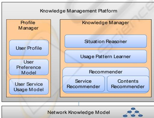
Figure 6: System Architecture of Knowledge Management Platform.
