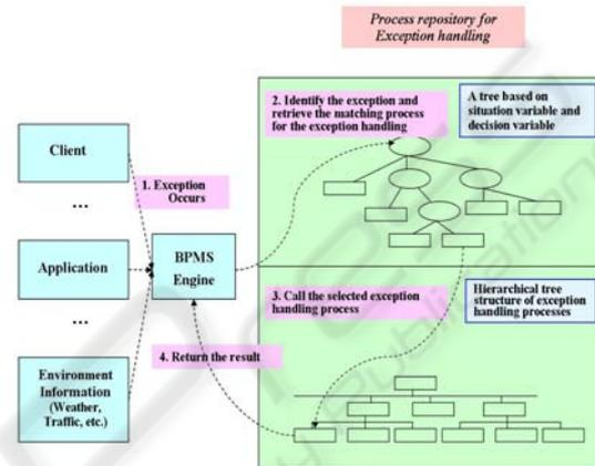
Figure 1: Architecture for exception handling process repository.
