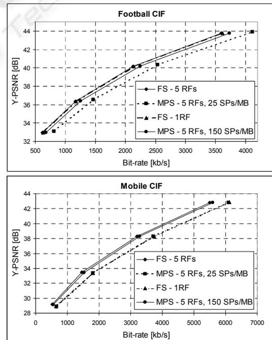
Figure 2: Rate-distortion curves for CIF sequences.
